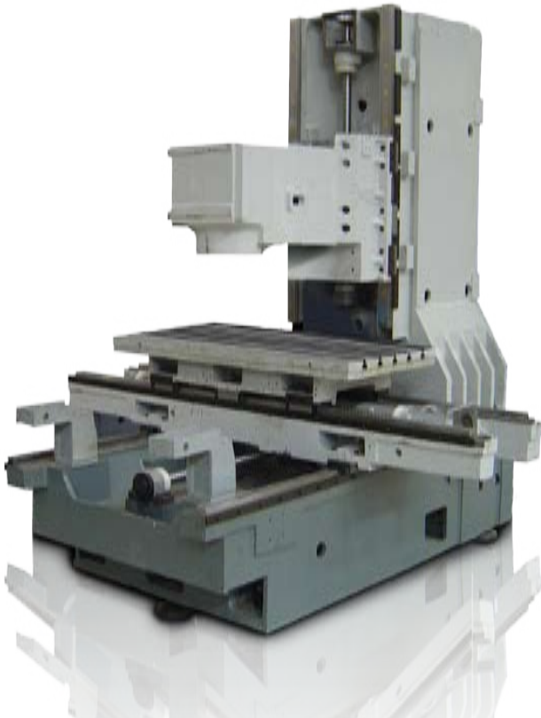
◀ Rugged structure of high quality, stress relieved casting and the thermosymmetrically arranged LM guide ways for chatter free precision machining under extreme working conditions
